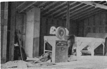
Slide 2 This is a view of one of the early mixers made up of three boxes, a screw, a scale and a leg for loading.
