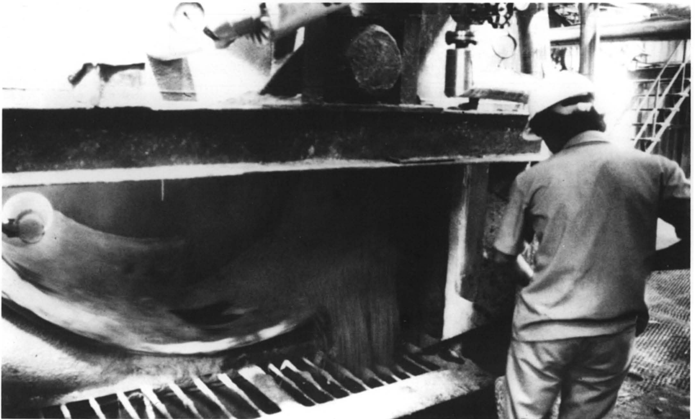
Figure 4. Drum Granulator in FPM Granulation Plant.
